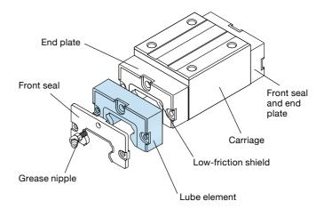
larly greased. It is not possible to refill the lube element. For ideal function the lube element should be replaced after 5 000 km of travel distance, unless regular greasing is given through the grease nipple.
